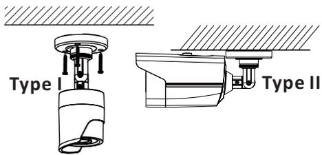
Figure 2-2 Fix the Camera to the Ceiling
