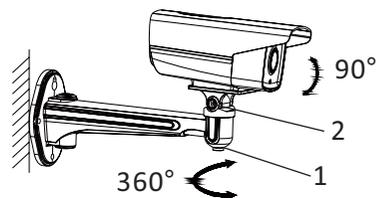
Figure 2-8 Angle Adjustment
