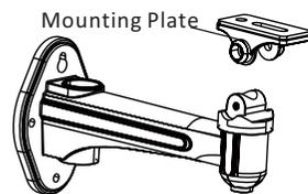
Figure 2-4 Disassemble Mounting Plate
