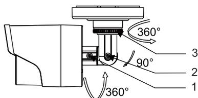
Figure 2-3 3-axis Adjustment
